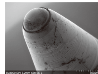
Accelerating voltage: 5 kV Image signal: SE Magnification: 60x Sample: Tip of ballpoint pen
