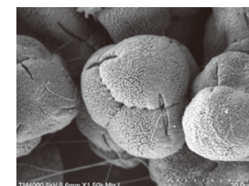
Accelerating voltage: 10 kV Image signal: Mixed image Magnification: 1,500x Sample: Azalea pollen Ionic liquid used
